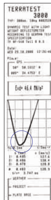
Picture 2: Test after 15 compaction drops by means of the light falling weight deflectometer on the same point. The test protocol shows one single displacement curve consisting of three congruent curves. The Evd value and the bearing capacity of the soil has increased of 20% compared to the first test.
