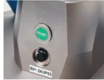
Control elements of the Bluetooth® sensor dome
