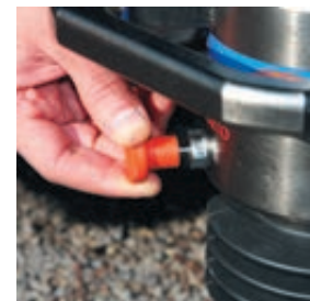
UNLATCHING THE TRANSPORTATION LOCK
