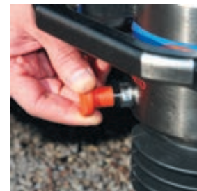
UNLATCHING THE TRANSPORTATION LOCK
