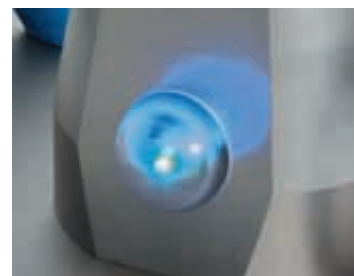
„Magic Eye“ BLUE: the connection is established
