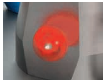
„Magic Eye“ RED: the sensor dome is ready for use and waiting for connection
