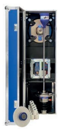
The Light Weight Deflectometer for dynamic load plate test is the perfect tool to test the compaction quality of unbound material in two minutes by only one person. The LWD gives you the possibility to check the ground soil before you start your construction to avoid damages of surface layers.
