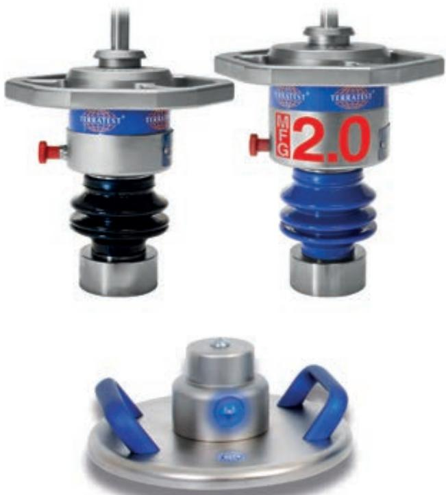
Light + Medium Heavy Weight Deflectometer with 10 kg/33lbs + 15 kg/33lbs for testing both: normal compaction and highly compacted layers (base courses) and soil improvements.
